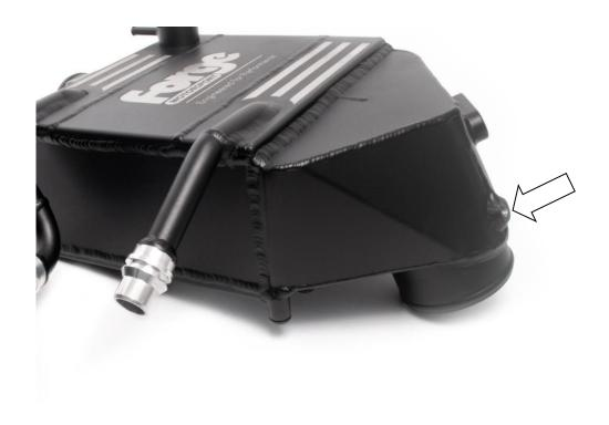
10. Ensure that the Chargecooler has been fully drained of coolant. Using a T30 Torx driver undo 5x screws and remove the 2x Mounting brackets from the OEM Chargecooler.
