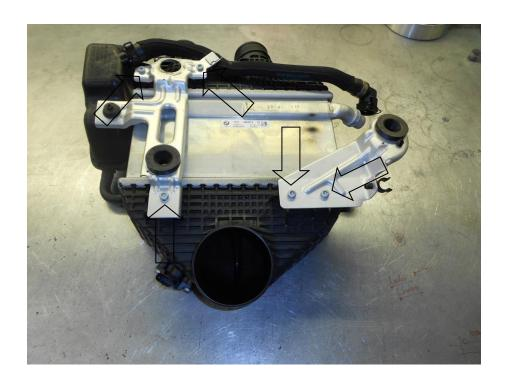
11. Refit the OEM mounting bracket to the Forge Chargecooler and secure in place with the remaining 5x Allen cap bolts M6 x 12mm and 6mm washer provided.
