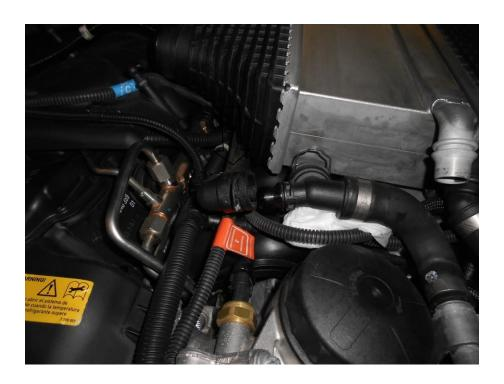
7. Pull the chargecooler up firmly to remove it from its 3x rubber mounts.
