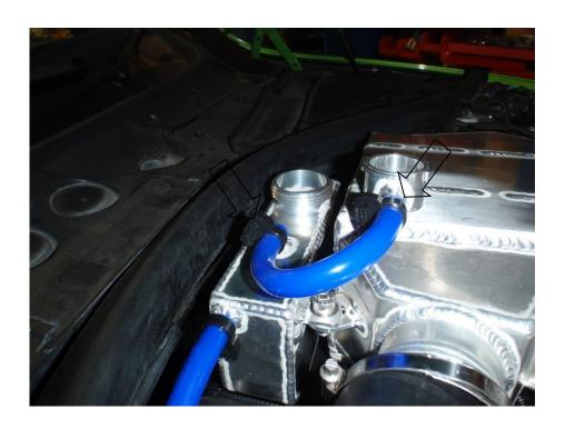
19. Carefully fill the Chargecooler with coolant and fit the radiator cap. Fill the expansion tank up to the level shown on the side glass window.
