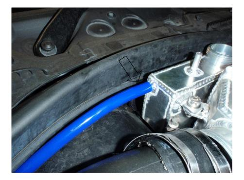
18. Using the remaining 8mm I/D Silicone x 170mm hose and 2x hose clamps connect the radiator neck to the expansion tank.
