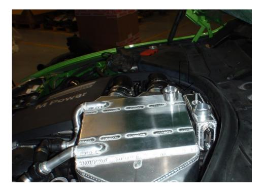
14. Reconnect the coolant feed and return pipes to the Chargecooler ensuring that the retaining clips are pushed into position.
