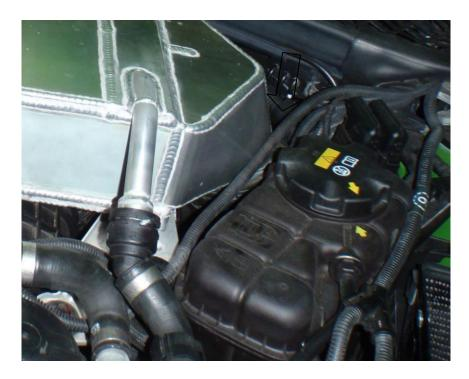
16. Remove the O-ring and retaining clip from the OEM expansion tank coolant coupler. Install the O-ring in the Forge blanking cap provided, attach this to the open coolant coupler and secure in position using the retaining clip.
