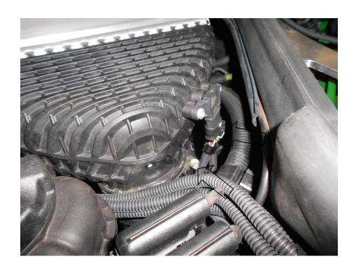
5. Pack a suitable absorbent material underneath the Chargecooler before using a flat blade screwdriver or similar tool to release the 2x retaining clips and pull the 2x couplers away from the Chargecooler.
