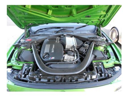
2. Pull the engine cover upwards to remove it from its mounts.
