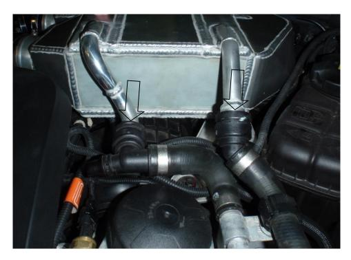
15. Using a suitable hose clamp driver tighten the single hose clamp at the Chargecooler outlet.
