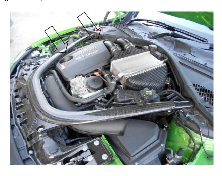
3. Using a 6mm hose clamp driver undo the 4x hose clamps and slide the hoses back over the boost pipes.
