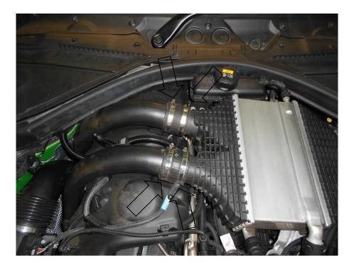
4. Disconnect the wiring to the MAP sensor and then use a 6mm socket or hose clamp driver to undo 1x hose clamp.
