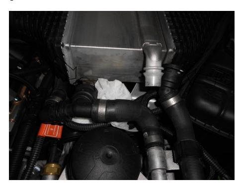
6. Release the 1x clip and disconnect the 1x hose from the coolant pipework.
