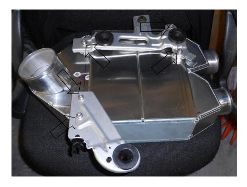
12. Lubricate the mounting bosses with a suitable lubricant (Silicone spray) and then fit the Chargecooler to the vehicle.
